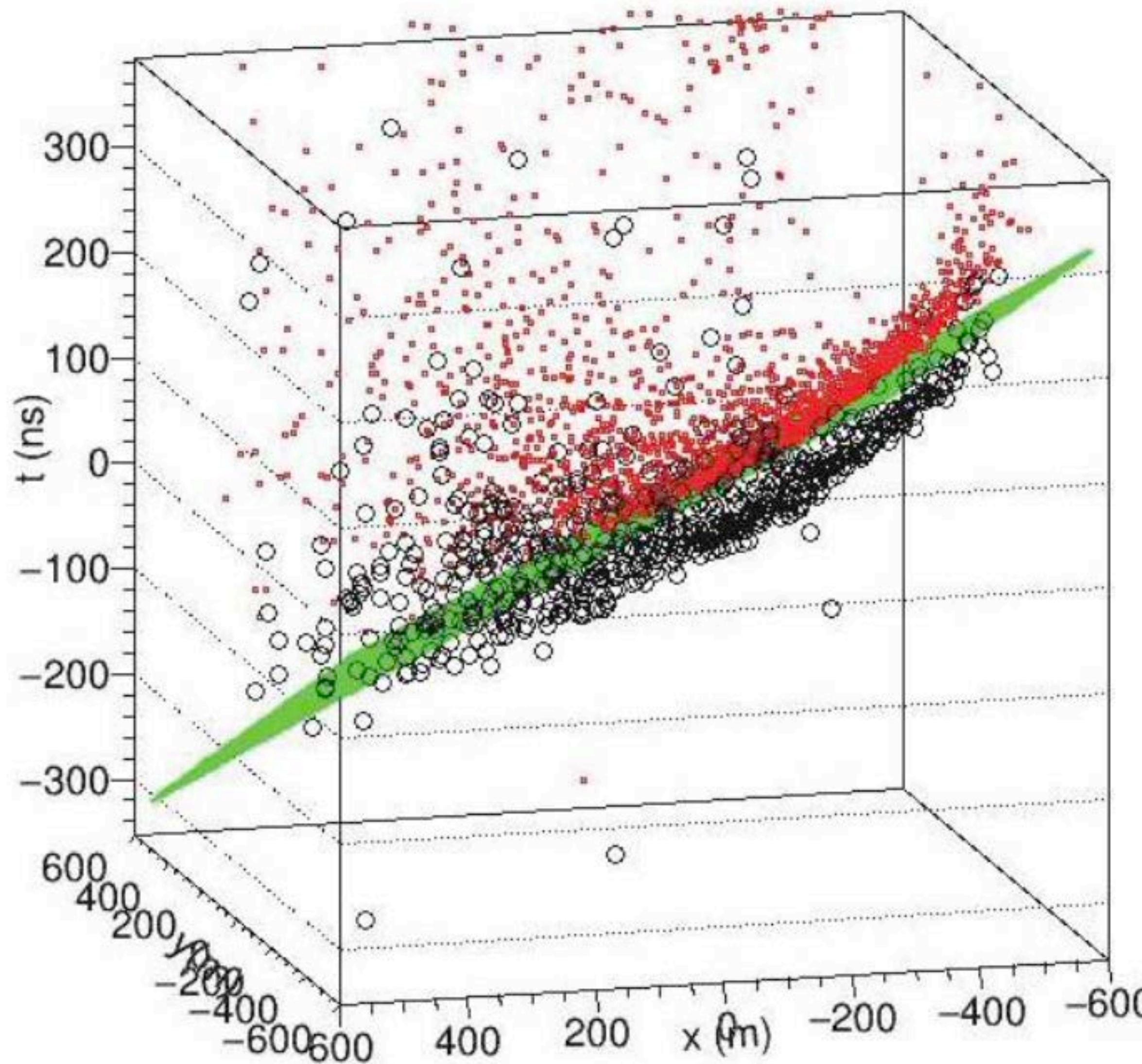
Secondary particles of an EAS detected by the ED array. The green plane is EAS front plane. The red squares are the fired ED. The black circles are the fired MD. The second front is caused by MD's dead time.
