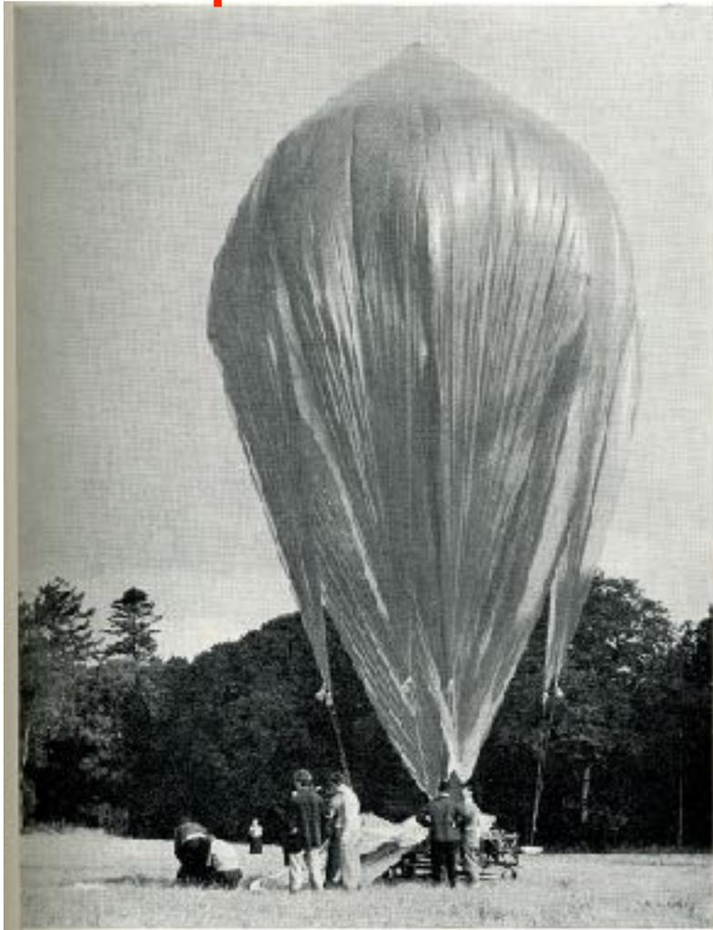
Fig. 7. Inflation of balloon of polyethylene just after dawn. The balloon has a total length of about 120 ft. and most of the fabric is on the ground. Such a balloon can in favorable conditions give level flight at about 90,000 ft. for many hours with a load of 40 kg.
