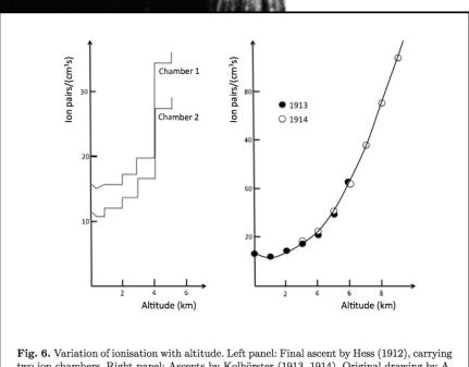
Fig. 6. Variation of ionisation with altitude. Left panel: Final ascent by Hess (1912), carrying two ion chambers. Right panel: Ascents by Körberster (1913, 1914). Original drawing by A. De Angelis.
