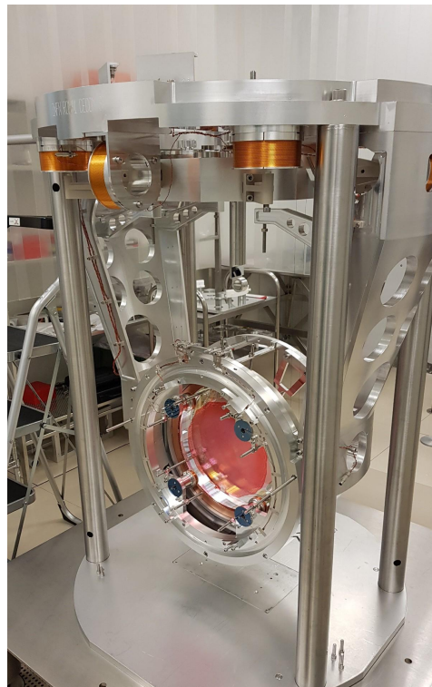
Mirrors weight 42 kgs to reduce the radiation pressure noise
