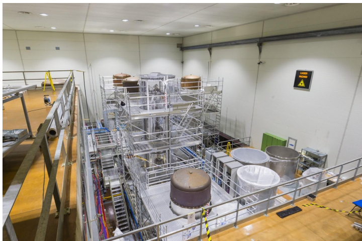
Superattenuators for seismic isolation
